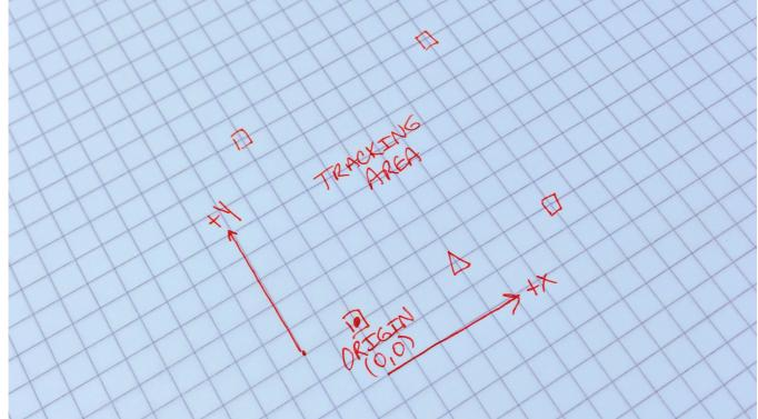
3. Survey anchor and master locations relative to the origin and desired XYZ axes. Measurements should be in meters.
