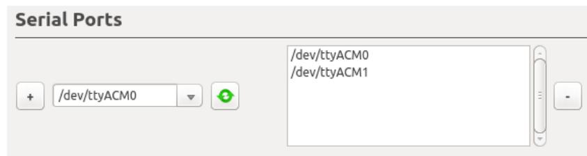
In the Serial Ports section, the dropdown box lists each location that is a possible USB device connection. This list can be updated by clicking the refresh button. All locations with which the CUWB Server will currently attempt to communicate are listed on the right side.
