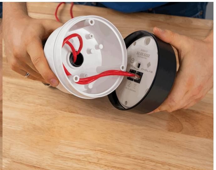
View of service loop
