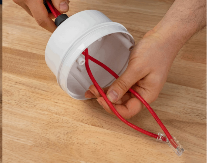
View of cable for service loop
